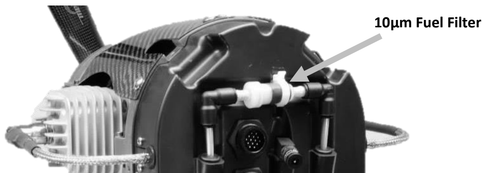
Figure 10. Fuel Filter Location
