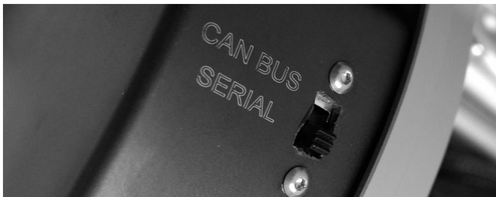
Figure 6: CAN BUS and Serial Switch
