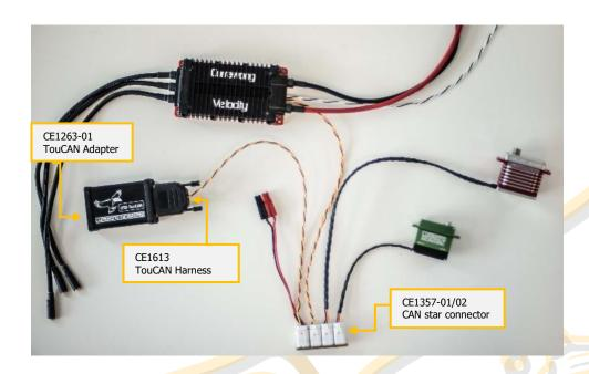
The TouCAN is a fully electrically isolated USB to CAN adapter for the integration and testing of in-situ CAN devices. The TouCAN provides advanced protection against ground shift and electrical noise, ensuring the safety of the host PC. It also provides optional bus termination for user convenience. Currawong offers a matching harness for the TouCAN.
