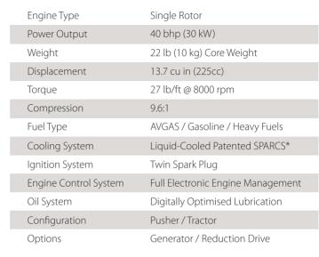
\*Self-Pressurising-Air Rotor Cooling System
